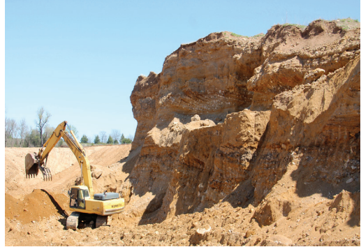
Figure 5. Buried valley filled with ice-contact stratified drift has been excavated as a source for sand and gravel for many years. South of Marysville and parallel to the Big Blue River valley.
